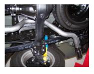
6. Install the overaxle tailpipe #E to the rear extension pipe #D. Use clamp #H to secure pipe. Do not tighten. Install hanger into rubber grommet.
