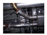
4. Install muffler onto headpipes 1.5"-2" with the louvers facing towards the converter. Use a jack stand to support the muffler. Use clamps #G to secure the muffler to the headpipe. Do not tighten. Muffler inlet is looking into the louvers.
