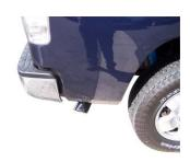
8. Install stainless steel tip. Clamp down. When you have everything in place, firmly tighten all bolts and clamps down securely. Use stainless steel cleaner and a Scotch Brite pad weekly to prevent tip from discoloration. Inspect all fasteners after 25-50 miles of operation and re-tighten as necessary. You may need to cut your stock tail pipe back to get your tip to fit correctly.
