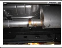
1.Remove from the first clamp located in front of the muffler.
