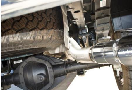
6. Install the exit pipe Item # B onto the over axle pipe. Do not tighten. Keep everything loose until you have proper clearance.
