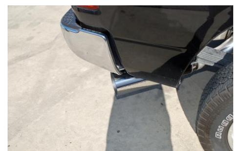
7. The system was designed to have the tip 1" below the quarter panel of the vehicle. With the tip in your desired position begin to tighten down all clamp connections from the front head pipe back. Clean tip before starting vehicle.
