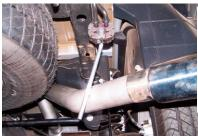
6. Install tail pipe #C into muffler 1 1/2" to 2". Use clamp #E to secure. Do not tighten. Insert welded hangers into rubber grommet
