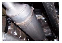
**4.** Install muffler #B onto head pipe #A 1 1/2"-2" with the louvers facing towards the converter. Use a jack stand to support the muffler. Use clamp #E to secure the muffler to the headpipe. Do not tighten. Muffler inlet is looking into the louvers. Outlet should be at the 10' O'clock position.
