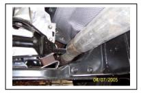
on to your existing stock support the converter. into rubber grommet. Do not tighten.
