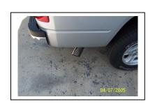
Install stainless steel tip. Clamp down. When you have everything in place, firmly tighten all bolts and clamps down securely. To clean stainless steel tip use any stainless steel cleaner.
