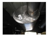
5. Install muffler #B onto head pipe #A  $1\frac{1}{2}$ "-2" with the louvers facing towards the converter. Use a jack stand to support the muffler. Use clamp #e to secure the muffler to the head pipe. Muffler outlet position will be about 3:00. Do not tighten. Muffler inlet is looking into the louvers.
