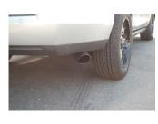
7. Install stainless steel tip. Clamp down. When you have everything in place with proper clearance of all brake lines, axle, etc... firmly tighten all bolts and clamps down securely. Use stainless steel or aluminum cleaner to polish tips. Inspect all fasteners after 25-50 miles of operation and re-tighten as necessary.
