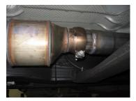
4. Install head pipe #A onto factory pipe. Use factory clamp to secure pipes together. Insert welded hanger into rubber grommet. Do not tighten.
