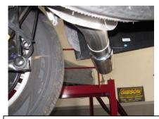
6. With proper clearance from spare tire install the exhaust tip onto the tailpipe. The system was designed to have the tip 1" below the quarter panel of the vehicle. With the tip in your desired position begin to tighten down all clamp connections from the
