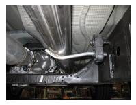
your existing stock flange and secure using the stock hardware. Do not tighten. Insert welded hanger into rubber grommet.
