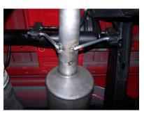
4. Slide the muffler #B into the headpipe at least 1.5"-2". Use a jack stand to support the muffler. Use clamp #E to secure muffler assembly to the headpipe. The outlet of the muffler will be at approximately 11 o'clock. The muffler inlet is looking into the louvers. Do not tighten.
