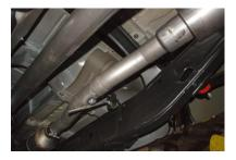
3. Install Headpipe # A onto the factory headpipe using the stock clamp. Do not tighten. Insert hanger into rubber grommet.
