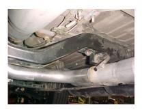
INSTALL Y-PIPE # A & I ONTO STOCK FLANGES USE YOUR STOCK HARDWARE TO SECURE. INSERT WELDED HANGER INTO RUBBER GROMMET, DO NOT TIGHTEN. USE CLAMP #J TO SECURE PIPES TOGETHER. DO NOT TIGHTEN.
