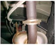
LAY OUT THE GIBSON EXHAUST ON THE FLOOR AND COMPARE PART #'S TO THE DRAWING. TO REMOVE YOUR FACTORY EXHAUST UN-BOLT YOUR TAILPIPE AT THE 2-BOLT FLANGE LOCATED BEHIND YOUR STOCK MUFFLER USE WD-40 TO AID YOU IN REMOVAL OF HANGERS FROM RUBBER GROMMETS. DO NOT DAMAGE THE GROMMETS,
