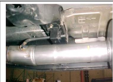
NEXT, INSTALL RESONATOR # B 1 1/2"-2" ONTO Y-PIPE USE CLAMPS # G TO SECURE PIPES TOGETHER, DO NOT TIGHTEN.
