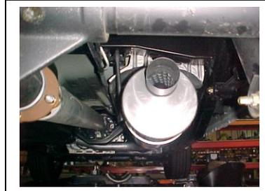
INSTALL MUFFLER # C ONTO YOUR RESONATOR 1 1/2" -2". USE CLAMP # G TO SECURE MUFFLER TO THE PIPE, DO NOT TIGHTEN. OUTLET WILL BE AT THE 12 O'CLOCK POSITION. INLET WILL BE LOOKING INTO LOUVERS.
