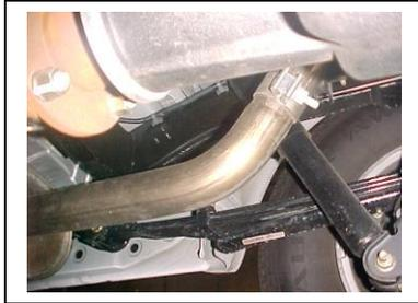
LAY OUT THE GIBSON EXHAUST ON THE FLOOR AND COMPARE PART #'S TO THE DRAWING. TO REMOVE YOUR FACTORY EXHAUST UN-BOLT YOUR TAILPIPE AT THE CLAMP LOCATED BEHIND YOUR STOCK MUFFLER USE WD-40 TO AID YOU IN REMOVAL OF HANGERS FROM RUBBER GROMMETS
