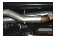
INSTALL HEADPIPE # A ONTO FACTORY PIPE. LINE UP THE NOTCH. USE CLAMP # G TO SECURE HEADPIPE TO FACTORY PIPE. DO NOT TIGHTEN. INSERT WELDED HANGER INTO RUBBER GROMMET.
