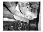
INSTALL DRIVER SIDE OVER AXLE TAILPIPE # D INTO MUFFLER 1½ TO 2". INSERT WELDED HANGER INTO RUBBER GROMMET, USE CLAMP # G TO SECURE PIPE TO MUFFLER. THIS PIPE WILL GO INTO THE DRIVERS SIDE OUTLET. DO NOT TIGHTEN
