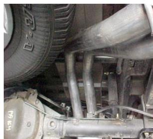
INSTALL PASS. SIDE TAILPIPE # E INTO MUFFLER 1 1/2"-2". USE CLAMP # H TO SECURE PIPE TO MUFFLER, DO NOT TIGHTEN.
