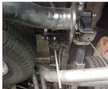
NEXT, INSTALL DRIVERS SIDE TAILPIPE # D INTO MUFFLER 1 1/2" -2". USE CLAMP # H TO SECURE PIPE TO MUFFLER, DO NOT TIGHTEN. INSERT WELDED HANGER INTO RUBBER GROMMET, BOLT TAILPIPES TOGETHER WITH
