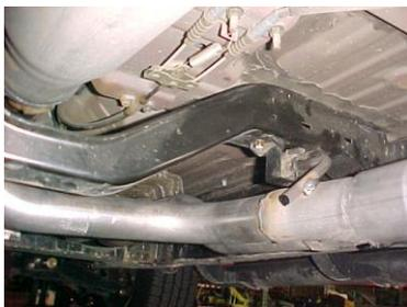
INSTALL Y-PIPE # A & L ONTO STOCK FLANGES USE YOUR STOCK HARDWARE TO SECURE INSERT WELDED HANGER INTO RUBBER GROMMET, DO NOT TIGHTEN. USE CLAMP # H TO SECURE PIPES TOGETHER. DO NOT TIGHTEN.
