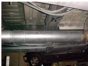
NEXT, INSTALL RESONATOR # B 1 1/2"-2" ONTO Y-PIPE USE CLAMP # G TO SECURE PIPES TOGETHER, DO NOT TIGHTEN.
