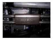
4. Install muffler #C onto headpipes 1.5"-2" with the louvers facing towards the converter. Use a jack stand to support the muffler. Use clamps #I to secure the muffler to the headpipes. Do not tighten. Muffler inlet is looking into the louvers.
