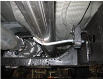
Next, install headpipe #A into the factory pipe. Insert welded hanger into the rubber grommet. Do not tighten
