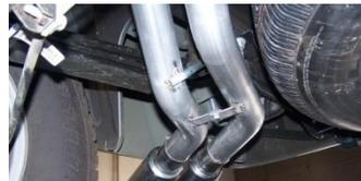
6. Now install driver side tailpipe #D. The spare tire may need to be loosened and pushed to the driver side to allow for clearance. Use bolt kit #H to attach both tailpipes together.
