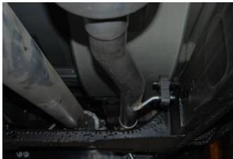
Next, install headpipe #A into the factory pipe. Insert welded hanger into the rubber grommet. Do not tighten
