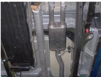
4. Install muffler #B with inlet towards Y-pipe. Use jack stands to support the muffler. Use clamp #F to secure the muffler to headpipe. Do not tighten. Muffler outlets will be level
