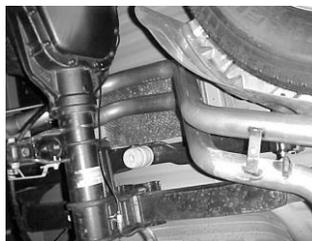
NEXT INSTALL DRIVERS OVER AXLE PIPE # D INTO MUFFLER 1 1/2 TO 2". USE CLAMP # F TO SECURE PIPE TO MUFFLER. DO NOT TIGHTEN. USE BOLT KIT # H TO SECURE PIPES TOGETHER. DRIVERSIDE TAB WILL BE ON THE BOTTOM.
