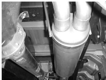
SLIP MUFFLER #B ONTO THE HEADPIPE 1 1/2" TO 2". THE OUTLETS WILL BE LEVEL. USE CLAMP #G TO SECURE MUFFLER TO HEADPIPE. DO NOT TIGHTEN.
