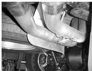
INSTALL PASSENGER SIDE OVER AXLE TAILPIPE # C INTO MUFFLER 1 1/2 TO 2". INSERT WELDED HANGER INTO RUBBER GROMMET, USE CLAMP # G TO SECURE PIPE TO MUFFLER. THIS PIPE WILL GO INTO THE PASSENGER SIDE OUTLET. DO NOT TIGHTEN
