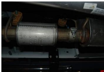
TO REMOVE YOUR STOCK EXHAUST, UNBOLT AND REMOVE IT FROM THE CLAMP LOCATED JUST BEHIND THE FACTORY RESONATOR. FOR EASIER REMOVAL OF THE FACTORY EXHAUST, CUT OFF THE STOCK TAILPIPE JUST BEHIND THE MUFFLER AND REMOVE. LEAVE ALL RUBBER GROMMETS ON THE HANGERS. USE WD-40 TO AID IN REMOVAL OF EXHAUST AND HANGERS.
