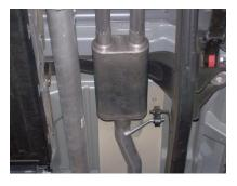
4. Install muffler #B with inlet towards Y-pipe. Use jack stands to support the muffler. Use clamp #F to secure the muffler to headpipe. Do not tighten.
