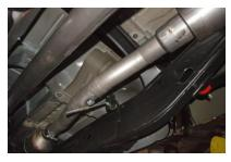
3. Install Headpipe # A onto use your factory clamp. Insert hanger into the rubber grommet. Do not tighten the clamp until install is complete.
