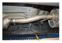
unbolt it at the clamp behind the Y-pipe. Make sure to leave all rubber grommets in the factory location. **You will reuse stock nuts and bolts.** For easier removal of exhaust, cut behind the muffler. Use WD-40 to remove hangers from grommets.
