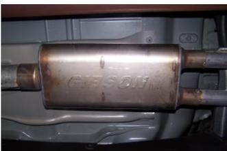
4. Slide muffler #B onto headpipe 1.5-2". Use a jack stand to support the muffler. Use clamp #F to secure the muffler to the headpipe. Do not tighten.
