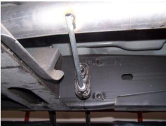
3. Install headpipe #A onto your existing stock front pipe and attach using stock hardware. Do not tighten. Insert welded hanger into rubber grommet.
