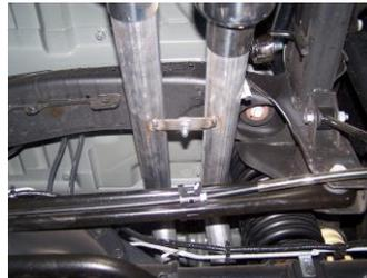
7. Use bolt kit #H to secure tailpipes together. (Driver side should be on the bottom.)
