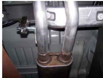
6. Slide the driver side over axle tailpipe #D into the muffler 1.5-2". Use clamp #G to secure tailpipe to muffler. Do not tighten. Insert welded hanger into rubber grommet.
