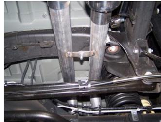
7. Use bolt kit #H to secure tailpipes together. (Driver side should be on the bottom.)
