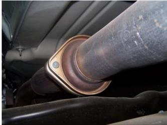
2. First remove hardware at the 2-bolt flange located in front of the muffler. Save the stock hardware as you will reuse it to attach new headpipe. Disengage the welded hangers from the OEM rubber grommets. Use WD-40 to aid in this process. Do not damage or remove the rubber grommets as you will reuse them to mount your new system. Now, cut off tailpipe and remove exhaust.
