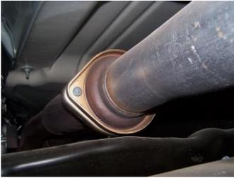
2. First remove hardware at the 2-bolt flange located in front of the muffler. Save the stock hardware as you will reuse it to attach new headpipe. Disengage the welded hangers from the OEM rubber grommets. Use WD-40 to aid in this process. Do not damage or remove the rubber grommets as you will reuse them to mount your new system. Now, cut off tailpipe and remove exhaust.
