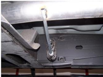
3. Install headpipe #A onto your existing stock front pipe and attach using stock hardware. Do not tighten. Insert welded hanger into rubber grommet.
