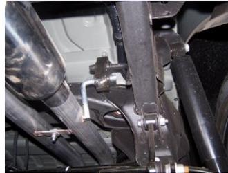
5. Slide the passenger side over axle tailpipe #C into the muffler 1.5-2". Use clamp #G to secure tailpipe to muffler. Do not tighten. Insert welded hanger into rubber grommet.
