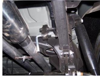
5. Slide the passenger side over axle tailpipe #C into the muffler 1.5-2". Use clamp #G to secure tailpipe to muffler. Do not tighten. Insert welded hanger into rubber grommet.
