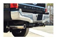
**8.** Install stainless steel tips. Clamp down. When you have everything in place, firmly tighten all bolts and clamps down securely. Use stainless steel cleaner weekly to prevent tip from discoloration. Inspect all fasteners after 25-50 miles of operation and re-tighten as necessary
