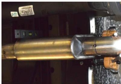
3. INSTALL MUFFLER # B. ONTO HEADPIPE 1 1/2" TO 2". USE CLAMP #E TO SECURE MUFFLER TO HEADPIPE. DO NOT TIGHTEN
