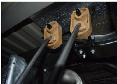
4. INSTALL OVERAXLE TAILPIPE # C INTO THE OUTLET OF THE MUFFLER 1 1/2" TO 2". INSERT WELDED HANGERS INTO THE FACTORY RUBBER GROMMET. USE CLAMP #E TO ATTACH THE OVERAXLE PIPE TO THE MUFFLER OUTLET. DO NOT TIGHTEN.
