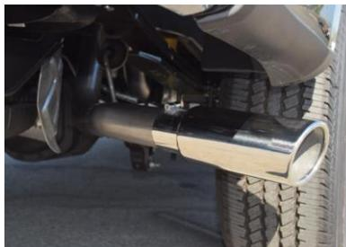
5. NOW INSTALL YOUR STAINLESS STEEL TIP. USE ANY ALUMINUM OR STAINLESS CLEANER TO POLISH YOUR TIP. THEN TIGHTEN ALL CLAMPS AND HANGERS.
