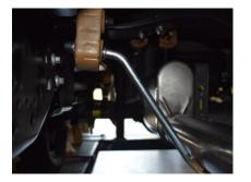
2. INSTALL HEADPIPE #A ONTO THE FACTORY PIPE. INSERT WELDED HANGER INTO RUBBER GROMMET. USE CLAMP #E TO ATTACH IT TO THE FACTORY PIPE. DO NOT TIGHTEN
