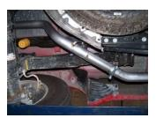
**4.** Install the passenger side overaxle tailpipe #C into the muffler 1½"-2". Use clamp #H to secure tailpipe to muffler. DO NOT TIGHTEN. Insert hanger into rubber grommets.
