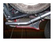
**7.** Next install the exit pipes #E. Use clamp #H to secure. DO NOT TIGHTEN.
