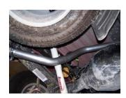
**6.** Install the driverside overaxle tailpipe #D into the muffler 1½-2". Use clamp #H to secure. DO NOT TIGHTEN. Rotate until it meets with the rubber grommet. DO NOT TIGHTEN.
