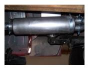
**3.** Install muffler #B onto head pipe #A  $1\frac{1}{2}$ "-2" with the louvers facing towards the converter and muffler outlets level. Use a jack stand to support the muffler. Use clamp #G to secure the muffler to the headpipe. Do not tighten. Muffler inlet is looking into the
