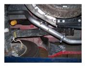
**4.** Install the passenger side overaxle tailpipe #C into the muffler 1½"-2". Use clamp #H to secure tailpipe to muffler. DO NOT TIGHTEN. Insert hangers into rubber grommets.
