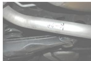
2. To remove the stock exhaust, measure 12" from the back of your stock muffler on both sides and cut. Do not discard your stock rubber grommets, for you will re-use them.
