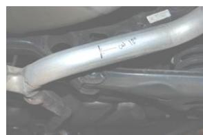
3. Install muffler assembly #A onto your existing passenger side pipe and attach with clamp #C. Do not tighten. Insert welded hanger into stock rubber grommet.
