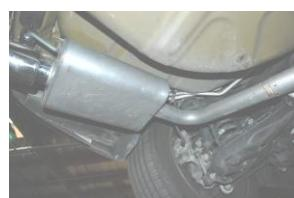
5. Adjust kit as needed. Tighten all clamps. Inspect all fasteners after 25-50 miles of operation and re-tighten as necessary.
