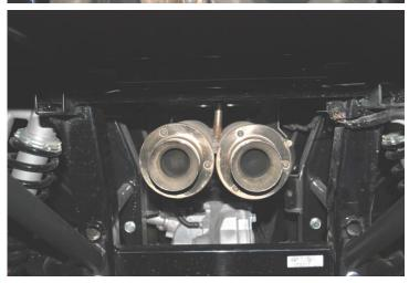
With the system securely in place in your desired position install the supplied clamp and tighten down the connection between the factory exhaust and the Gibson exhaust. It is important with this style clamp you place it to the edge of the Gibson pipe.
