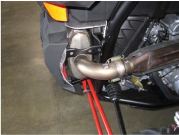
2. Once you have removed the heat shield loosen the factory brackets. Keep loose until final install.
