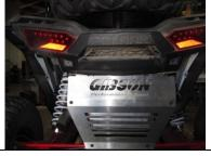
4. Install rear Gibson beauty plate. Use the factory bolts to install. Once they have been installed tighten the Gibson brackets at the rzr frame. Adjust plate for a level finish.
