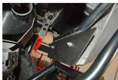
3. Next install Item # F and Item # B. You will use the supplied bolts to bolt both plates together. The polished rear plate will be on the outside of the vehicle and Item # F is the heat shield on the inside of the rear valance designed to protect the rear plastics.
