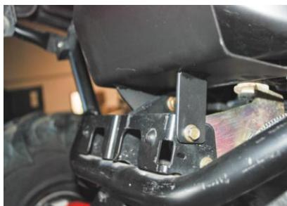
2 Install Item #G your air box heat shield. You will use the factory bolts that hold your rear differential on. Once installed re tighten bolts.
