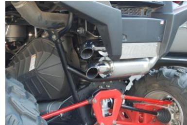
6. Install Item #A slide the hangers in factory mounts from the passenger side until lined up with the header. Once you have it lined up re install the factory springs.
