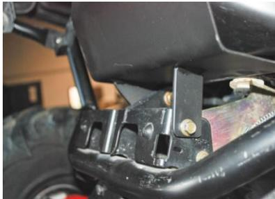
2 Install Item #G your air box heat shield. You will use the factory bolts that hold your rear differential on. Once installed re tighten bolts.
