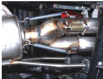
7. With the header still loose, but the header bolts installed attach the supplied Gibson springs. Use the Needle nose pliers and a small flat head screw driver to assist with the install. It is important to use your safety goggles.
