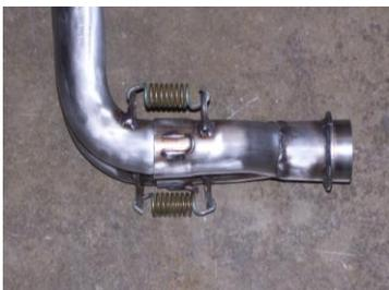
5. Use the factory springs to attach Item C to the header pipes. Item C the collector will have a top and a bottom. When looking at the collector from the side one way will have the single exit facing up wards at about a 10 degree angle or down ward. You want the single exit of the collector facing downward when slipping it onto the header pipes.
