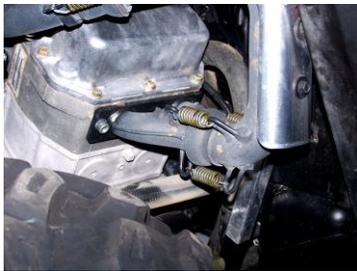
2. Next remove the entire exhaust. Do not damage the factory springs or Exhaust gaskets as they will be re used.
