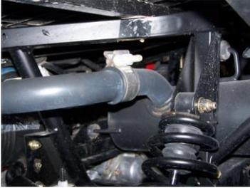
1. Remove the factory muffler by using the 15mm wrench or socket at the band clamp shown in the photo. Spraying a small amount of WD-40 will help with the removal of muffler from the rubber hangers
