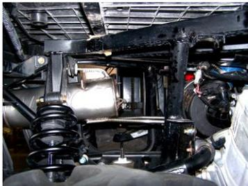
3. Now install Gibson Muffler Item D. Slip the muffler in from the rear of the RZR. Slip the lower long hangers into the rubber grommets first then pull back and slide the upper hanger into the single rubber grommet.
