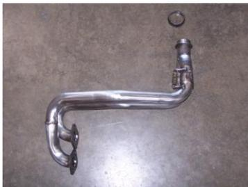
4. You will need to assemble the header and collector before installing onto the RZR. Item A will be installed onto the front exhaust port. While Item B is the rear exhaust port.
