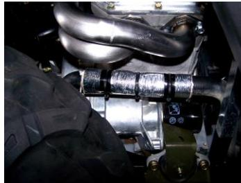
8. After springs are installed make sure everything is fitting properly and tighten the header bolts. Now install the supplied heat wrap around the radiator hose seen in the photo.
