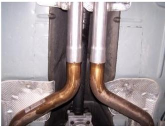
2. To remove the stock exhaust, first you must remove the factory cross member under the X pipe. Then unbolt and remove driver side tailpipe at the flange. Now unbolt and cut tack welds on factory clamps at the X pipe and carefully remove factory exhaust, save clamps for new exhaust installation. The 2.75" clamps are included in case you can't use the factory clamps. Leave all rubber grommets on hangers. Use WD-40 to help remove hangers.
