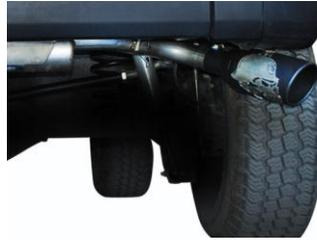
4. Install Metal Mulisha tips. Clamp down. When you have everything in place, firmly tighten all bolts and clamps down securely. Inspect all fasteners after 25-50 miles of operation and re-tighten as necessary.
