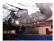
2.Remove the whole exhaust from the clamps (located just after your factory headers). To make it easier, remove the support in the *middle* of the car. Do Not Disgard. You will reinstall.
