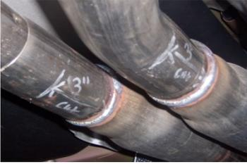
2. To remove stock exhaust, measure 3" from stock resonator & cut. Do not damage or remove the rubber grommets as you will re-use them to mount your new system.
