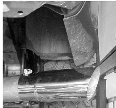
INSTALL THE STAINLESS STEEL TIP TO YOUR DESIRED LOOK. USE ANY ALUMINUM OR STAINLESS STEEL CLEANER TO POLISH YOUR TIP. TURN VEHICLE ON AND CHECK FOR LEAKS. NOW TIGHTEN ALL CLAMPS AND MAKE SURE ALL HANGERS ARE IN THE CORRECT PLACE.
