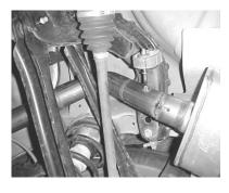
INSERT THE WELDED HANGER ON EXTENSION PIPE INTO THE RUBBER GROMMET.
