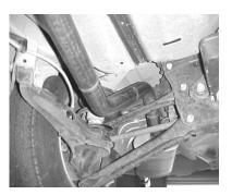
INSTALL REAR EXTENSION PIPE # B, USING CLAMP # F TO ATTACH TO RESONATOR.
