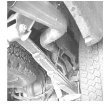
**INSTALL OVERAXLE** TAILPIPE #B AND ATTACH TO MUFFLER **OUTLET USING HANGER #D, WHEN INSTALLING** THE TAILPIPE YOU WILL NEED TO JACK THE BODY OF THE VEHICLE UP, TO SLIDE THE TAILPIPE THROUGH THE LEAF SPRING AND THE BOTTOM OF THE FRAME. ALSO THE SHOCK IN FRONT OF THE AXLE MAY NEED TO BE DISCONNECTED AND LOWERED TO SLIP THE TAIL PIPE IN. INSERT THE WELDED HANGER INTO THE RUBBER GROMMETT.
