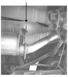
NEXT, INSTALL REAR MUFFLER HANGER #D AND INSERT INTO RUBBER GROMMETT. DO NOT TIGHTEN.
