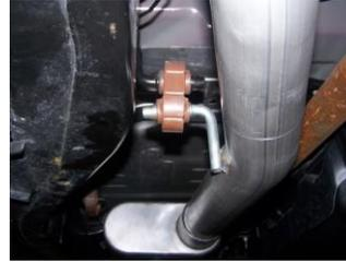
**4.** Install overaxle tailpipe #C into the muffler 1½"-2". Insert welded hanger into rubber grommet. Use clamp #F to secure tailpipe to muffler. **DO NOT TIGHTEN**
