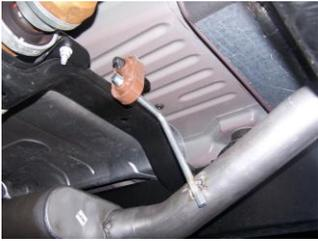
**2.** Install head pipe #A onto your existing stock front pipe and attach using stock bolts. **DO NOT TIGHTEN.** Insert welded hangers into rubber grommet.
