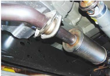
TO REMOVE YOUR STOCK EXHAUST, REMOVE IT FROM THE 2 BOLT FLANGE LOCATED JUST IN FRONT OF THE MUFFLER AND REMOVE HANGERS FROM RUBBER GROMMETS BY PULLING EXHAUST TOWARDS THE REAR OF THE VEHICLE, USE WD-40 TO AID IN REMOVAL, LEAVE GROMMETS IN PLACE.
