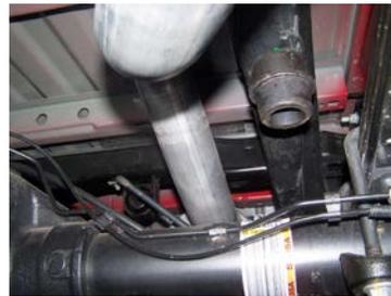
INSTALL OVERAXLE TAILPIPE #C INTO MUFFLER 1 ½" TO 2". INSERT HANGERS INTO RUBBER GROMMETS. USE CLAMP #E TO SECURE PIPE TO MUFFLER. DO NOT TIGHTEN.
