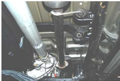
INSTALL HEADPIPE # A INTO STOCK PIPE. THE END OF THE PIPE SHOULD BE AT THE 12 O'CLOCK POSITION., INSERT WELDED HANGERS INTO RUBBER GROMMET. ATTACH WITH BOLT KIT #F. DO NOT TIGHTEN. REMOVE THE HANGER FROM THE FRAME & RELOCATE TO THE HOLES JUST TO THE LEFT OF THE OTHER HOLES YOU WILL NEED TO PRY THE INSERTS OUT & RE-INSTALL SEE PHOTO
