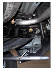
**5.** Next, install the exit pipe #D. Use clamp #F to secure to the tailpipe. DO NOT TIGHTEN. Insert welded hanger into rubber grommet.
