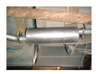
Install muffler onto head pipe 1-1/2" to 2" with the louvers facing towards the converter. Use a jack stand to support the muffler. Use clamp #G to secure the muffler to the head pipe. Do not tighten. Muffler inlet is looking into the louvers.
