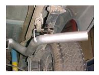
Install the exit pipe #D on to the tailpipe. Insert welded hanger into the rubber grommet. Secure together with clamp #G. Do not tighten. Roll the exitpipe until it is at the correct
