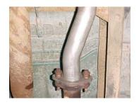
Install head pipe #A into flange #F. Bolt the flange and headpipe to the stock flange. Do not tighten.
