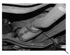
**UN-BOLT STOCK HEADPIPE** JUST BEHIND THE CATALYTIC CONVERTER. **DO NOT DAMAGE** STOCK BOLTS AND **GASKET! FOR YOU WILL NEED TO RE-USE** THEM. CUT OFF YOUR STOCK TAILPIPE JUST BEHIND THE MUFFLER AND REMOVE. LEAVE ALL RUBBER GROMMETS ON THE HANGER. USE WD-40 TO HELP WITH REMOVAL OF STOCK EXHAUST AND HANGERS.
