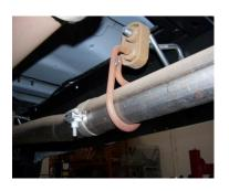
1. LAY OUT THE EXHAUST SYSTEM SO IT MATCHES THE DRAWING. MAKE SURE ALL PART NUMBERS ARE CORRECT. UNBOLT THE WELDED MUFFLER ASSEMBLY IN FRONT OF THE MUFFLER. DO NOT REMOVE THE EXTENSION PIPE BEHIND THE CONVERTER. FOR AN EASIER REMOVAL OF THE FACTORY EXHAUST. CUT THE TAILPIPE JUST BEHIND THE FACTORY MUFFLER. LEAVE ALL RUBBER GROMMETS IN PLACE. USE WD-40 FOR EASIER REMOVAL OF FACTORY HANGER.
