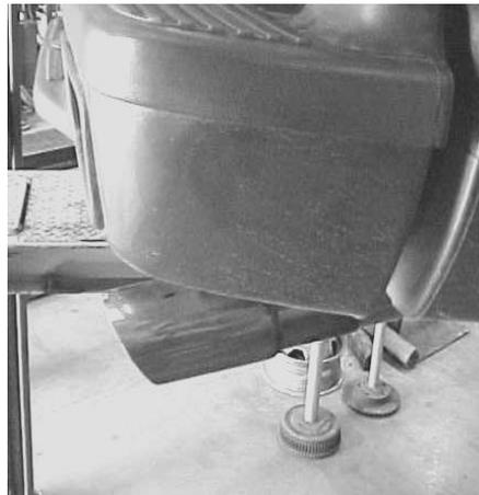
INSTALL YOUR STAINLESS STEEL TIP. USE ANY ALUMINUM OR STAINLESS STEEL CLEANER TO POLISH YOUR TIP. THEN TIGHTEN ALL CLAMPS AND HANGERS.
