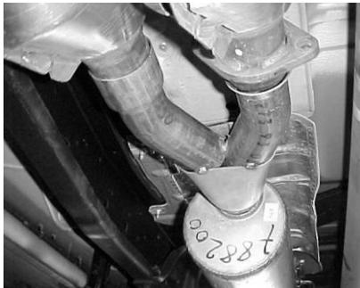
INSTALL MUFFLER ASSEMBLY #A. REUSE DRIVERSIDE HEADPIPE GASKET & APPLY SMALL AMOUNT OF HI-TEMP GASKET SEALER. BOLT DRIVERSIDE FLANGE & REUSE FACTORY BOLTS. ATTACH THE PASSENGER SIDE HEADPIPE USING CLAMP #E. DO NOT TIGHTEN
