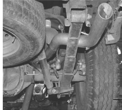
INSTALL OVERAXLE TAILPIPE #B INTO MUFFLER. INSERT WELDED HANGER INTO FACTORY RUBBER GROMMET. CLAMP DOWN WITH HANGER #D TO MUFFLER. DO NOT TIGHTEN
