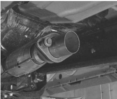
INSTALL FLANGE #G ONTO HEADPIPE #A. ATTACH TO FACORY FLANGE RE-USIEING FACTORY BOLTS TO INSTALL IT. SNUG UP THESE BOLTS.
