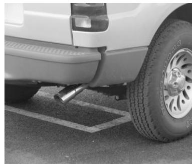
ROTATE TAILPIPE UNTIL YOU HAVE A MINIMUM OF 1" FROM ALL PIPES, RUBBER BRAKE LINES, TIRES, SWAY BAR, SHOCKS, ETC. THEN TIGHTEN ALL CLAMPS AND HANGERS. REINSTALL THE REAR SHOCK MOUNT. INSTALL YOUR STAINLESS STEEL TIP TO YOUR DESIRED LOOK. USE ANY ALUMINUM OR STAINLESS STEEL CLEANER TO POLISH YOUR TIP.
