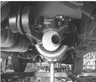
SLIDE MUFFLER #B ONTO HEADPIPE 1 1/2" TO 2". USE CLAMP #E TO SECURE MUFFLER TO HEADPIPE. DO NOT TIGHTEN. OUTLET SHOULD BE AT THE 3 O'CLOCK POSITION. MUFFLER INLET IS LOOKING INTO LOUVERS.
