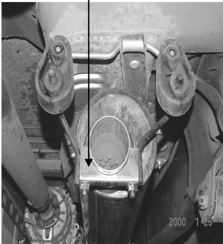
NEXT, INSTALL O.E REAR HANGER #D. DO NOT TIGHTEN. INSTALL TAILPIPE #B, WHEN INSTALLING THE TAILPIPE YOU WILL NEED TO JACK THE BODY OF THE VEHICLE UP TO SLIDE THE TAILPIPE THROUGH THE LEAF SPRING AND THE BOTTOM OF THE FRAME. ALSO THE SHOCK IN FRONT OF THE AXLE MAY NEED TO BE DISCONNECTED AND LOWERED TO SLIP THE TAIL PIPE IN. INSERT WELDED HANGER INTO RUBBER GROMMETT.
