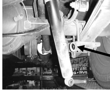
FOR AN EASIER INSTALLATION OF THE OVERAXLE PIPE DISCONNECT THE LOWER REAR SHOCK MOUNT.
