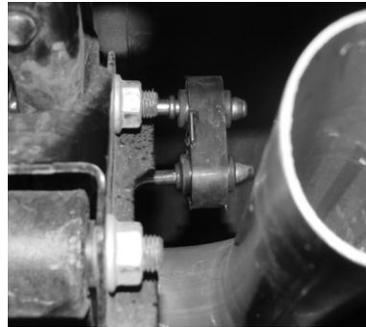
SLIP THE OVERAXLE PIPE #C THROUGH THE LEAF SPRING IN BETWEEN THE SHOCK AND THE SWAY-BAR AND INTO THE MUFFLER AT LEAST 1 1/2" NO MORE THAN 2" USE HANGER #E TO CLAMP PIPE TO MUFFLER.
