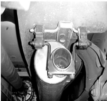
ONCE THE MUFFLER AND HEADPIPE ARE INSTALLED ROTATE THE MUFFLER AND HEADPIPE UNTIL MUFFLER OUTLET IS POSITIONED AT 3 O'CLOCK AND SITTING LEVEL UNDERNEATH THE VEHICLE. INSTALL THE O.E. HANGER #E ONTO OUTLET OF MUFFLER AND INSERT WELDED HANGERS INTO DIAPHRAGM GROMMET
